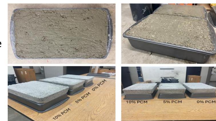
Concrete- PCM samples with 0%, 5% and 10%
